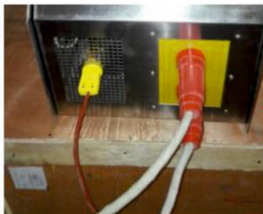
Connect the coil and thermocouple to machine
